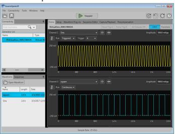
SourceXpress is a PC based software environment that enables Tektronix waveform creation plug-ins, simulates the native environment of a Tektronix AWG70000 or AWG5200 series Arbitrary Waveform Generator, and provides control of a connected generator. SourceXpress allows you to create signals anywhere without being tied to a signal generator. SourceXpress brings a uniform look and feel to waveform creation while enabling an ever growing library of waveform creation plug-ins.
