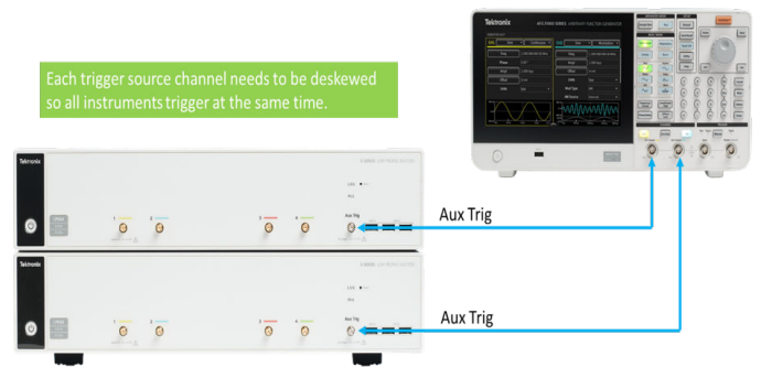
Setup diagram to quickly achieve moderate skew among channels
