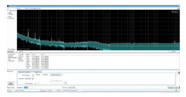
The RSA7100A's intrinsic phase noise of -134 dBc/Hz, at this frequency and across its operating range, provides ample measurement margin for a vast majority of applications.
