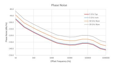
The previous figure shows the RSA7100A typical and nominal phase noise performance.
