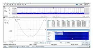
Shown above is a 700 MHz wide chirped signal. A time overview is presented at the top of the display that shows the pulses in the current acquisition. Phase deviation is displayed on the left, showing the characteristic parabolic shape of a frequency chirp. The signal has variations in repetition interval, shown in both the pulse table and the spectrogram on the right.
