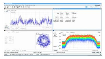
In the illustration above, a 5 GHz carrier modulated with 500 MSymbols/sec pi/4-QPSK is analyzed with the RSA7100A Option B800 and SignalVu-PC application license SVMH. A measurement summary, EVM vs. Time, and constellation display are shown along with the continuous monitoring of the DPX spectrum.
