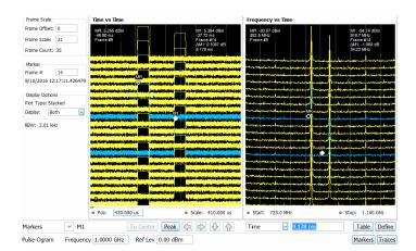
The illustration above is the unique Pulse-Ogram display in SignalVu-PC application license SVPH. This is a waterfall of triggered pulses showing their relationship to the trigger in time domain. Variations are immediately seen as changes in timing vs. trigger. Each time domain trace is represented as a spectrum on the right side of the display for immediate correlation of time and frequency domain effects.
