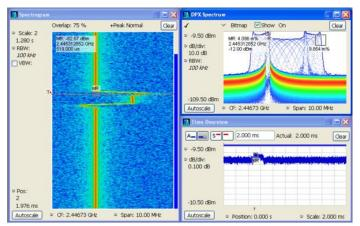
Trigger and Capture: The DPX Density<sup>™</sup> Trigger monitors for changes in the frequency domain, and captures any violations into memory. The spectrogram display (left panel) shows frequency and amplitude changing over time. By selecting the point in time in the spectrogram where the spectrum violation triggered the DPX Density<sup>™</sup> Trigger, the frequency domain view (right panel) automatically updates to show the detailed spectrum view at that precise moment in time.
