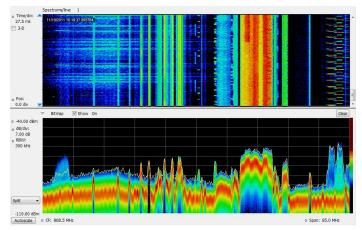
DPX Spectrograms provide gap-free spectral monitoring for up to days at a time. 60,000 traces can be recorded and reviewed, with resolution per line adjustable from 125 µs to 6400 s.
