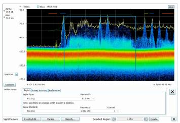
In this illustration, a single region has been selected. Since we have declared this to be an 802.11g signal, the spectrum mask for the 802.11g signal is shown overlaid in the region. The signal is a close match to the spectrum mask, However we can see some interferences with some likely Bluetooth signals in the ISM band
