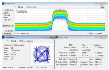
Time-correlated views in multiple domains provide a new level of insight into design problems not possible with conventional analyzers. Here, modulation quality and the constellation measurements are combined with the continuous monitoring of the DPX <sup>®</sup> spectrum display.
